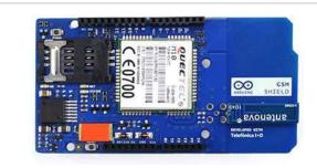
Figure 4: GSM shield is used along with the microcontroller.
