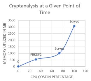
Figure 3. Graph showing the CPU Cost Vs Memory utilized at certain time.
