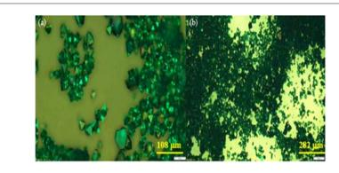
Figure 3. Optical microscopical images of Cu-BTC Metal organic framework at different magnifications.
