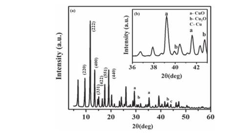
Figure 1. X-ray diffraction pattern of Cu-BTC metal organic framework (inset shows the expanded view).
