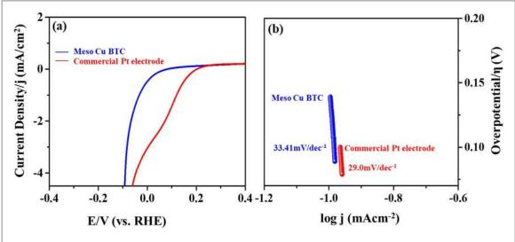
Figure 8. (a) LSV steady-state polarization plots of Meso CuBTC and Pt electrode and (b) Tafel plot for Meso Cu-BTC and Pt electrode in 1 M NaOH.
