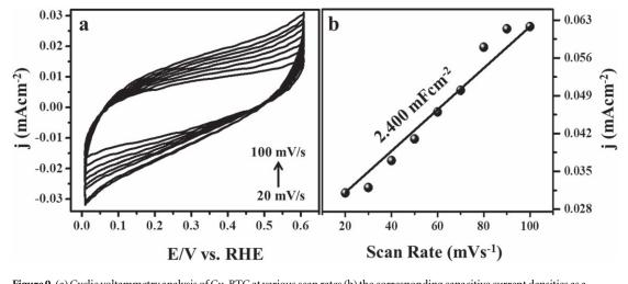
Figure 9. (a) Cyclic voltammetry analysis of Cu-BTC at various scan rates (b) the corresponding capacitive current densities as a function of scan rate.
