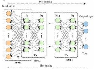
FIGURE 3. The Architecture of DBN.
