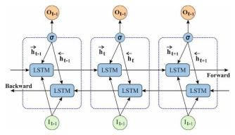
FIGURE 2. The Structure of Bi-LSTM.
