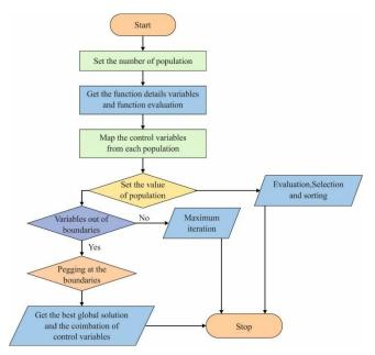
FIGURE 4. The Flowchart of BMO algorithm.
