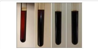
Figure 4: The degraded crude oil- Biodiesel mixture for varying mixing ratios (left to right:- 1:2 sample,1:1 sample,2:1 sample,blank sample).
