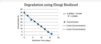
Figure 5: Plot of concentration against time for degradation of crude oil in Elengi biodiesel.
