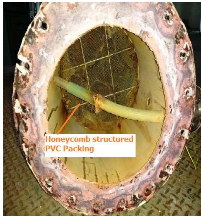
Figure 3. Photograph of the humidifier with honeycomb PVC packing
