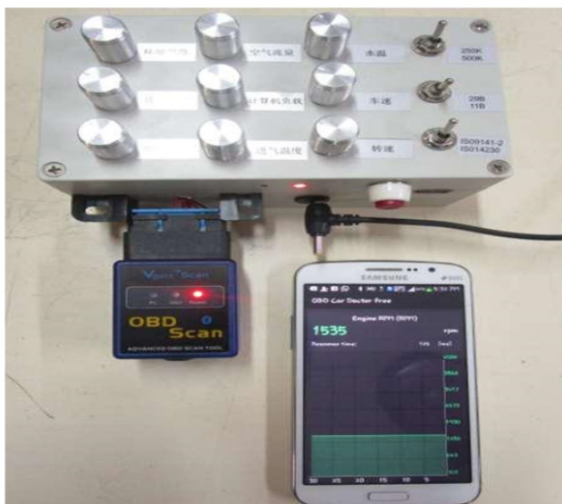
Figure 11. Engine RPM value is displayed on the LCD.
