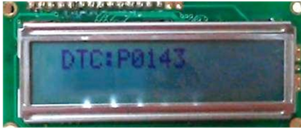
Figure 10. DTC is displayed on the LCD.
