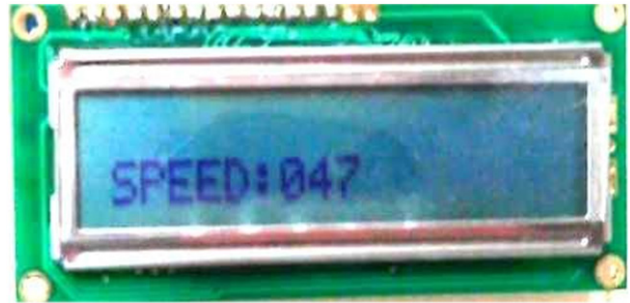
Figure 7. Vehicle's speed value is displayed on the LCD.
