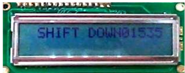
Figure 9. Shift Down is displayed on the LCD.
