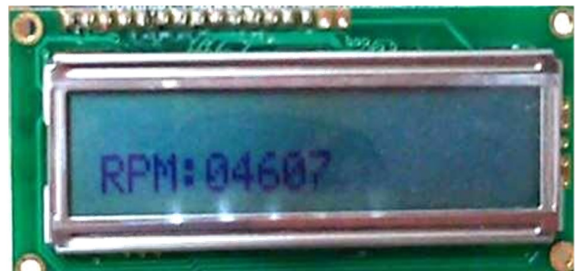
Figure 8. Engine RPM value is displayed on the LCD.
