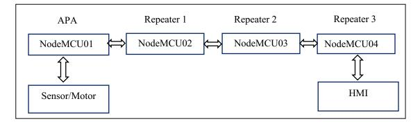
Figure 7. Basic structure of Long-range topology.
