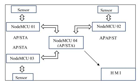
Figure 3. Basic structure of star topology.
