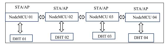
Figure 5. basic Structure of Radial topology.
