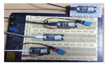
Figure 13. Wireless networking with radial topology.
