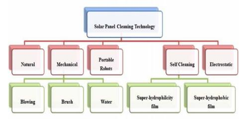
Figure 1. Solar PV panel cleaning methods.
