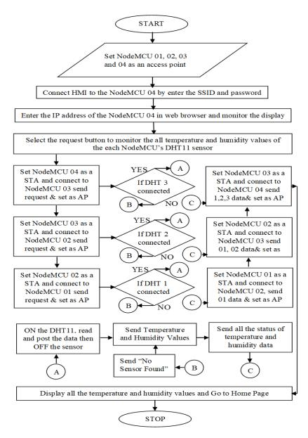
Figure 6. Flow chart of Radial topology
