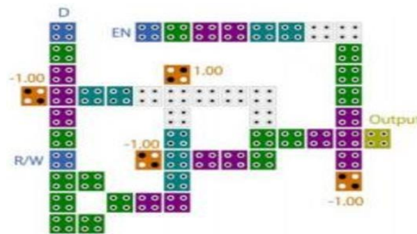
Figure 7. QCA layout of a memory cell
