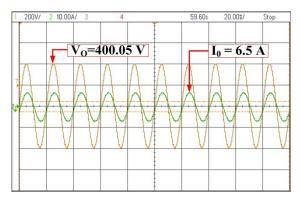
FIGURE 30. 15MLI experimental waveforms with non-linear load (Motor load).
