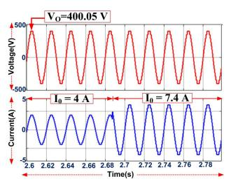
FIGURE 25. The output waveform of 15MLI with R to L load.
