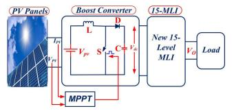
FIGURE 1. Proposed system configuration.
