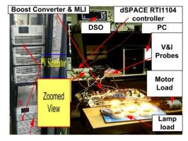
FIGURE 34. Prototype model of 15MLI.
