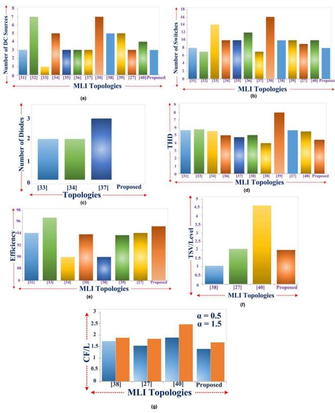
FIGURE 39. Components comparison with Recent MLIs. (a) N<sub>SDC</sub>, (b) N<sub>SW</sub>, (c) N<sub>D</sub>, (d) THD, (e) Eff, (f) TSV, (g) C.F/Levels.
