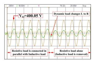
FIGURE 32. 15MLI experimental waveforms with non-linear to a linear load
