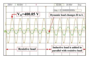
FIGURE 31. 15MLI experimental waveforms with linear to a non-linear load.
