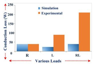
FIGURE 35. Conduction losses of 15MLI.
