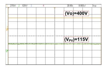
FIGURE 4. Experimental output waveforms of Converter & Solar PV.
