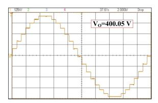
FIGURE 28. 15MLI experimental output waveform.
