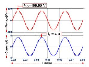
FIGURE 23. The output waveform of 15MLI with two cycles.
