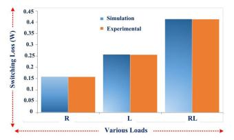
FIGURE 36. Switching losses of 15MLI.
