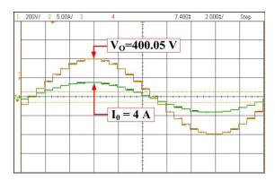
FIGURE 29. 15MLI experimental waveforms with linear load.
