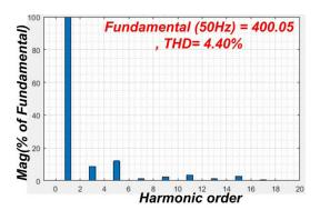
FIGURE 27. 15MLI THD Simulation of 15MLI.
