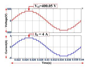
FIGURE 22. The output waveform of 15MLI with one cycle.
