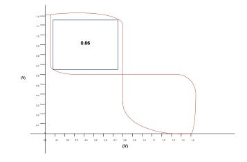
Figure 5. Static Noise Margin (SNM) of 8T SRAM cell.
