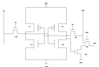
Figure 1. Conventional 8T SRAM cell
