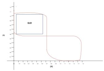
Figure 6. Static Noise Margin (SNM) of 6T SRAM cell
