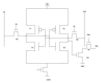
Figure 2. Power Gating Implementation in 8T SRAM cell
