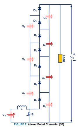
$V_0$  is the output voltage of the converter which is the product of the number of levels N and the capacitor voltage Vc is
