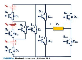
Bridge produces a positive level of voltage. The output voltage level is  $+3V_{dc}$  i.e., +400 volts.
