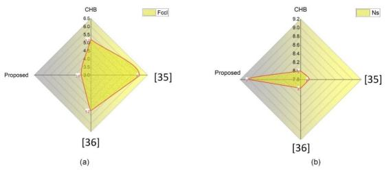
FIGURE 23. (a) Comparison of components count per level of proposed MLI with other topologies.
