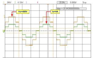
FIGURE 8(b). Experimental output voltage and current waveforms of a five-level inverter
