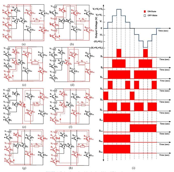
FIGURE 10. Modes of operation of the developed 7-Level MLI topology
