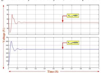
FIGURE 3. The 4-level converter & FC Simulation waveforms
