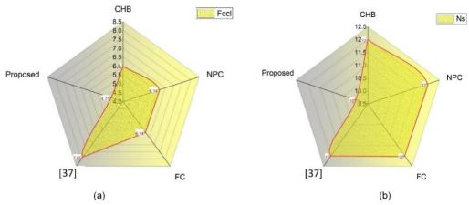
FIGURE 24. (a) Comparison of components count per level of proposed MLI with other topologies.
