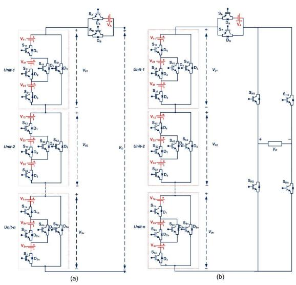
FIGURE 5.1. Developed Cascaded Multilevel Inverter.
