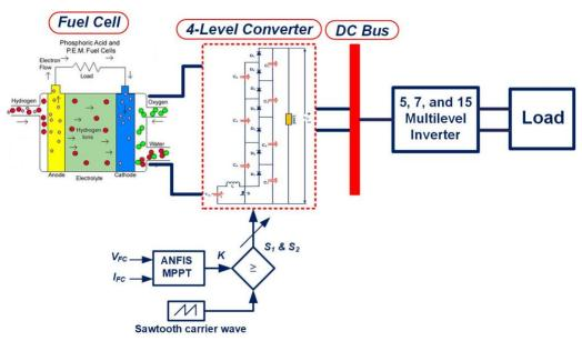
FIGURE 1. Proposed Topology with Fuel cell stack
