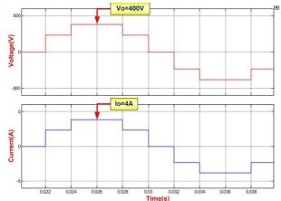
FIGURE 8(a). Simulation output voltage and current waveforms of a fivelevel inverter
