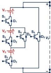
FIGURE 5. Developed Fundamental unit
