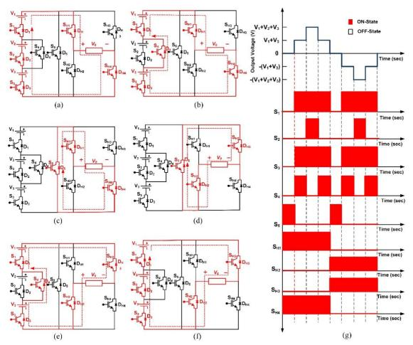
FIGURE 7. Modes of operation of the developed 5-Level MLI topology
