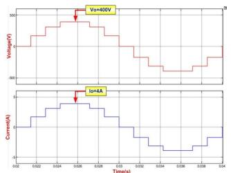
FIGURE 11(a). Simulation output voltage and current waveform of Seven-level inverter
