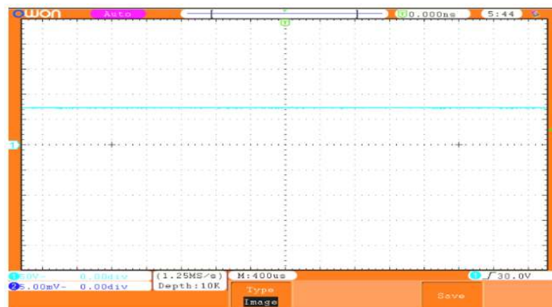
Figure 20. Generated voltage of SRG with filter.
