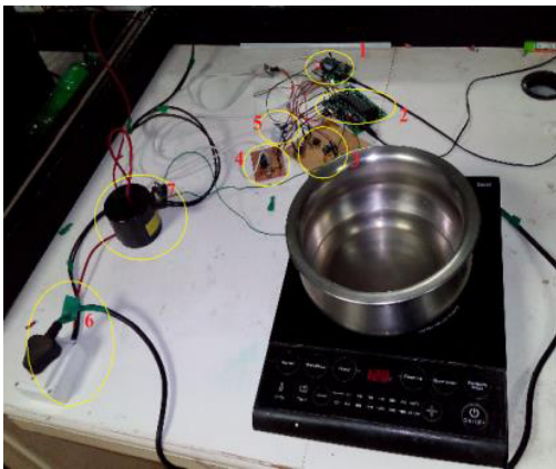
Fig. 7. Hardware setup of low standby power socket with smart meter
