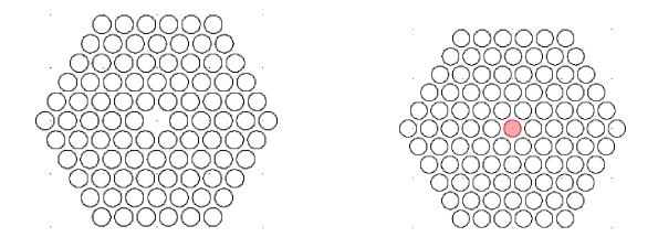
FIGURE 1. (a) Schematic diagram of the silica core PCF with air hole diameter d and Period  $\Lambda$ ; (b) Liquid core PCF consisting CS2 or nitrobenzene at the core region
