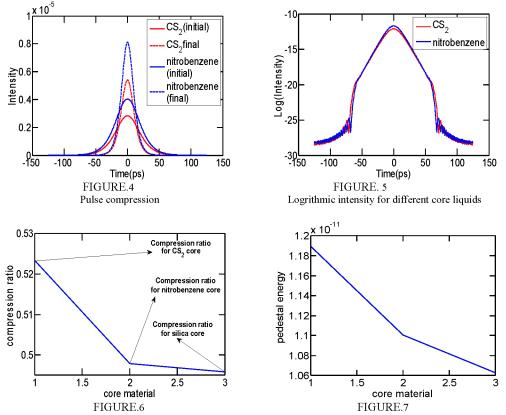
Compression ratio and Pedestal energy for different core material where 1, 2 and 3in the x axis for CS<sub>2</sub>, nitrobenzene and silica respectively
