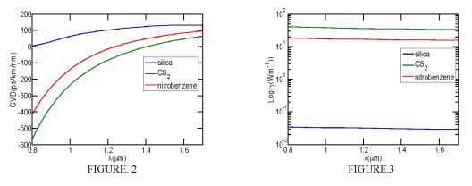
Variation of dispersion (Fig.2) and nonlinearity (Fig.3) for different core materials
