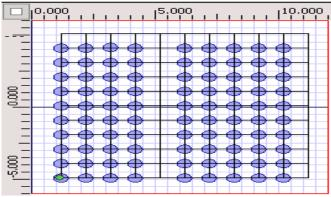
Fig. 3: A line defect of removed column of rods
