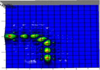
**Fig. 5:**  $90^{\circ}$  Bend Waveguide with biofluid of refractive index (n = 1.37)
