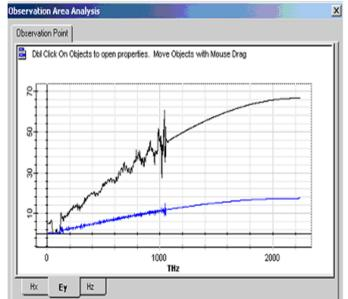
Fig: 7: Electric field intensity as function of frequency for 90<sup>0</sup> bends waveguide with and without biofluid.
