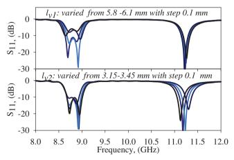
**FIGURE 4** The antenna performance with change in parameters  $l_{v1}$  and  $l_{v2}$
