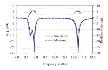
**FIGURE 7** The dual-band antenna performance:  $S_{11}$  and realized gains
