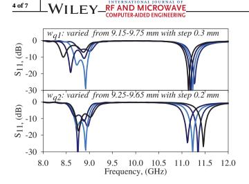
**FIGURE 5** The antenna performance with change in parameters  $w_{q1}$  and  $w_{q2}$
