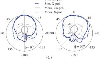
**FIGURE 8** The radiation patterns at frequencies of A, 8.72, B, 8.92 and C, 11.25 GHz in two principle cut planes
