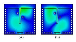
**FIGURE 3** Absolute electric field on the top metallic layer at the frequencies. A, 8.92 GHz and B, 11.24 GHz
