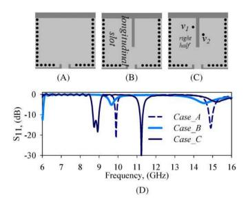
**FIGURE 2** A, HMSIW cavity (case\_A). B, HMSIW with a longitudinal slot (case\_B). C, Proposed design with loaded vias (case\_C). D, Performance at antenna evolution stages. HM, half-mode; SIW, substrate integrated waveguide
