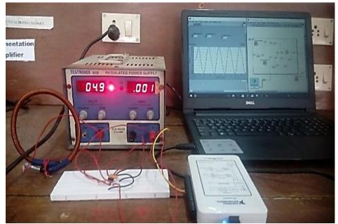
Fig. 2: Hardware Setup of Rogowski Coil.
