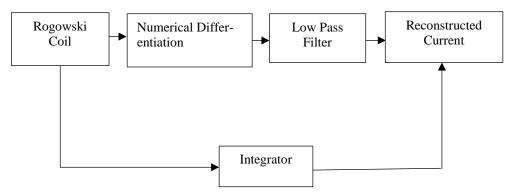
Fig. 1: Block Diagram Representation of Reconstruction Methods.
