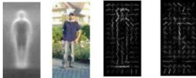
Fig. 2. HOG detectors cue mainly on silhouette contours (especially the head, shoulders and feet). (a) The average gradient image over the training examples; (b) A test image; (c, d) The R-HOG descriptor weighted by respectively the positive and the negative SVM weights. Image Courtesy: Navneet Dalal 23
