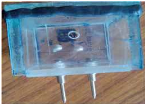
Figure 5. Prototype gas test cell.
