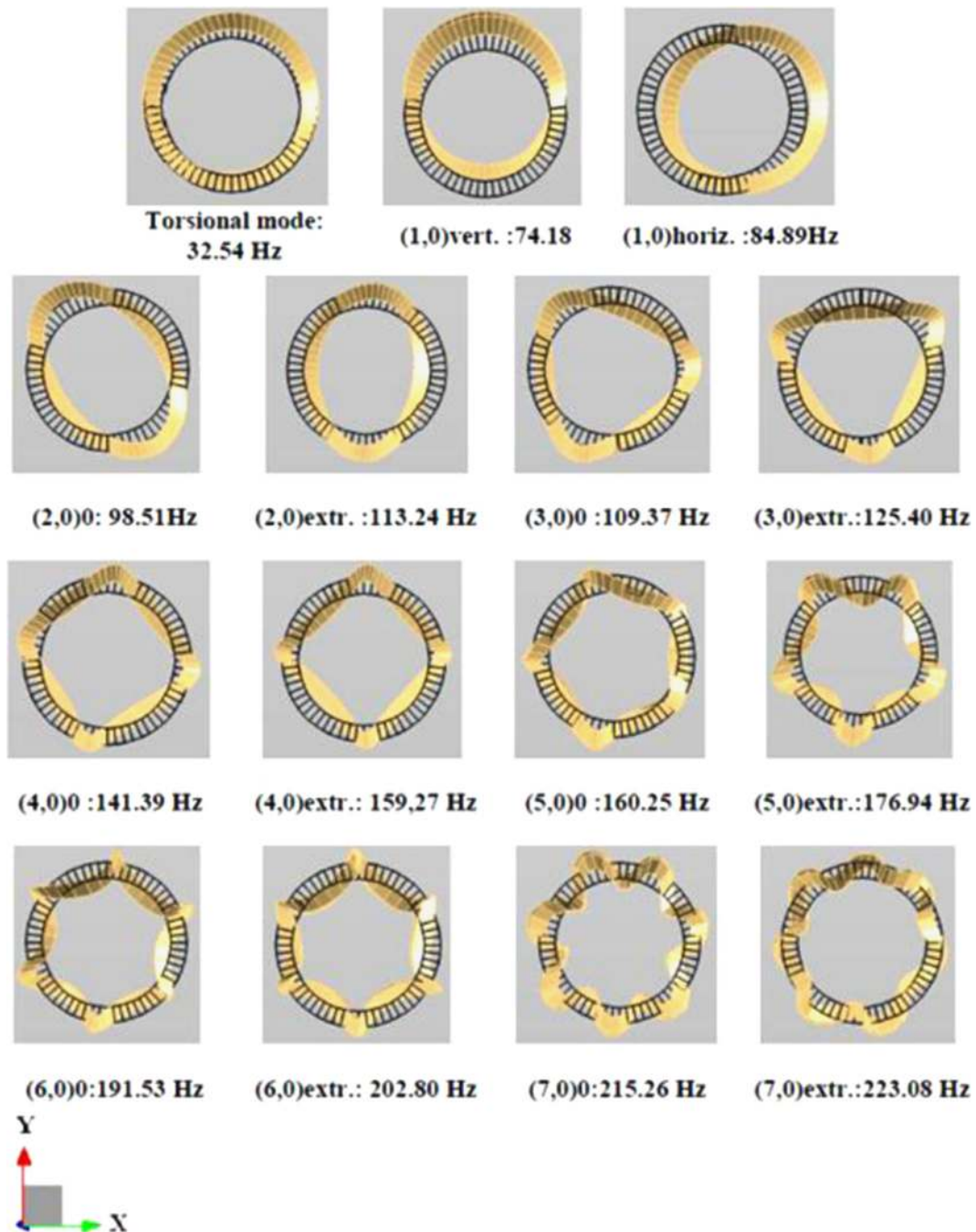
Fig. 11. Operational modal parameters obtained from straight cleat impact test.
