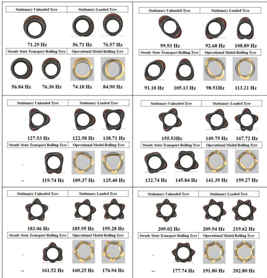
Fig. 16. Mode shape comparison among various tyre conditions.
