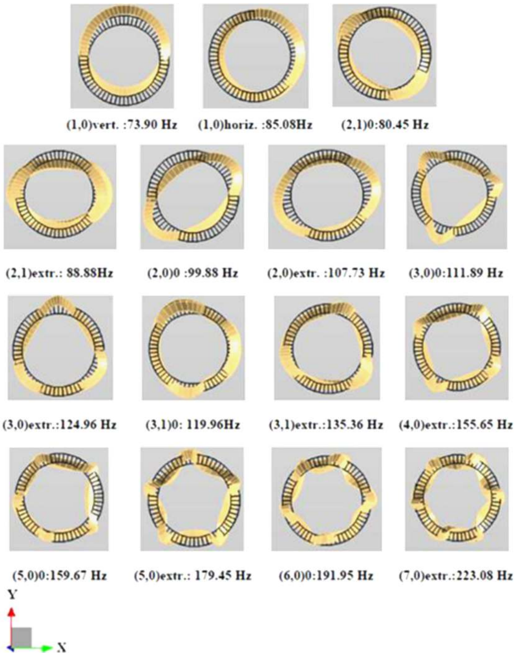
Fig. 12. Operational modal parameters obtained from 45° inclined cleat impact test.
