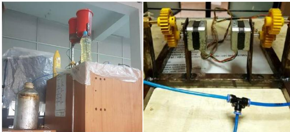
Figure 4. Mounted fuel tank systems and the stepper motor arrangement
