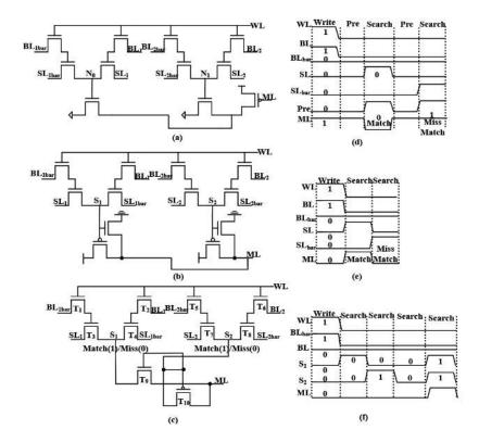
**Figure 3.** DCAM cells and timing diagram of their operational phases: a) 5T DCAM design for two bits; b) PF-DCAM design for two bits; c) proposed PF-DCAM designs for two bits; d) precharge type DCAM operational phases; e) precharge free type PF-DCAM operational phases; f) proposed precharge free-type PF-DCAM operational phases.
