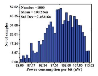
Figure 8. Performance metrics of the proposed CAM on 1000 runs of MC simulation: histogram of power consumption.
