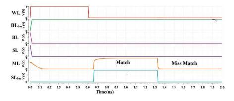
Figure 6. Transient response of proposed CAM design.
