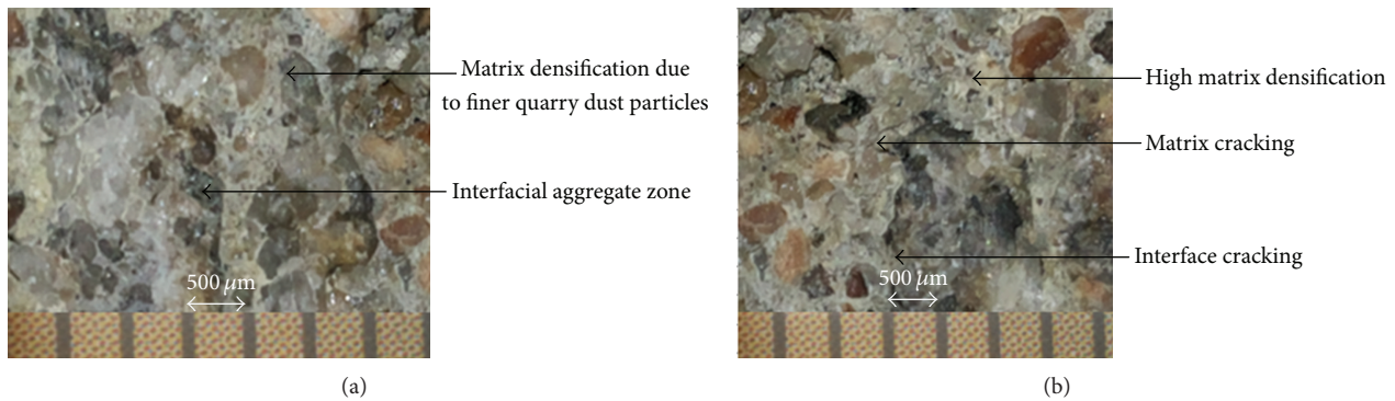
FIGURE 12: (a) Microscopic view of quarry dust concrete without stress (50x magnification). (b) Microscopic view of quarry dust concrete at 40% load (50x magnification).
