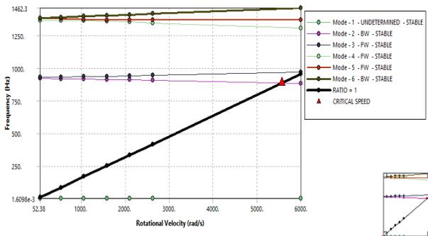
Figure 5. Campbell diagram of FG shaft
