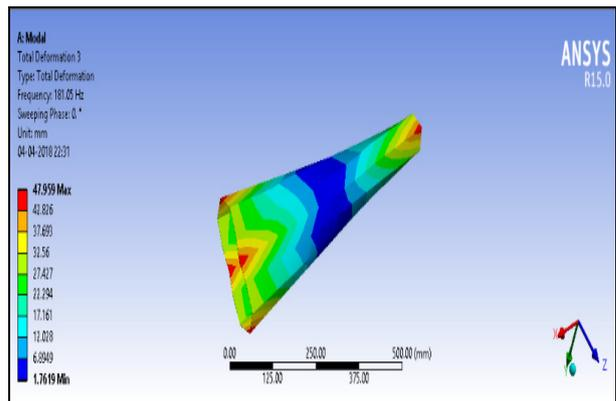
Figure 8. Third mode shape - conventional steel shaft
