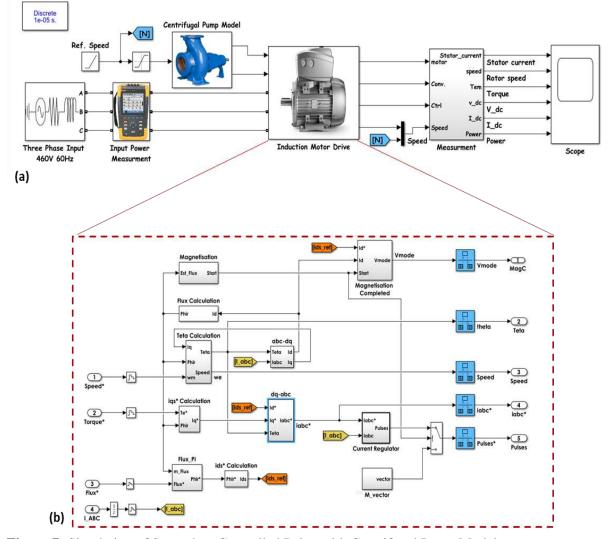
**Figure 7:** Simulation of Sensorless Controlled Drive with Centrifugal Pump Model *a*) Overall simulation model b) Sensorless vector control of induction motor drive
