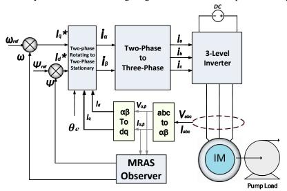
Figure 6: Schematic of Sensorless Controlled Pump Drive
