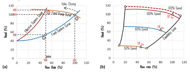
Figure 2. Centrifugal pump operation (a) variable speed and (b) fixed speed
