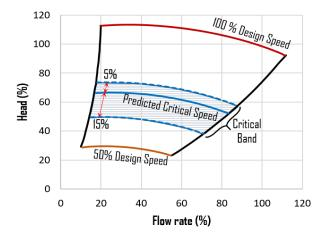
Figure 5. Critical speed band curve
