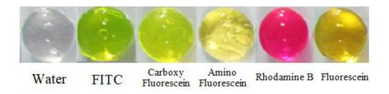
Figure 2: SPA bead absorption with 5 different fluorescent compounds with water as a control.
