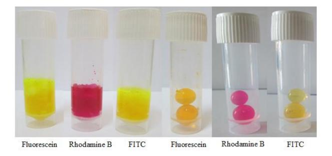
Figure 1: The three fluorescent compounds absorption in SPA powder verses SPA bead.
