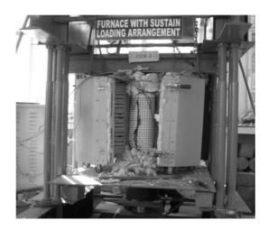
Figure 1. Set-up of furnace with sustained loading arrangement.
