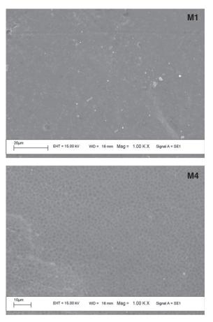
Fig. 1. SEM photographs of the top surface of membranes formed from 82.5 (M1) and 85% (M4) of NMP in 17.5 and 15% of PES respectively, magnification 1000.
