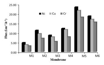
**Fig. 7.** Solvent effect and solvent composition in PES membranes on permeate rate (flux) of Cu(II), Ni(II) and Cr(III) metal ions with PDDA microligand.
