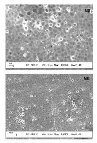
**Fig. 2.** SEM photographs of the top surface of membranes formed from 85% of DMSO (M5) and DMF (M6) as solvents in 15% PES polymer, magnification 1000.
