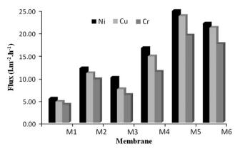
**Fig. 6.** Solvents effect and solvents composition in PES membranes on permeate rate (flux) of Cu(II), Ni(II) and Cr(III) metal ions with PVA microligand.
