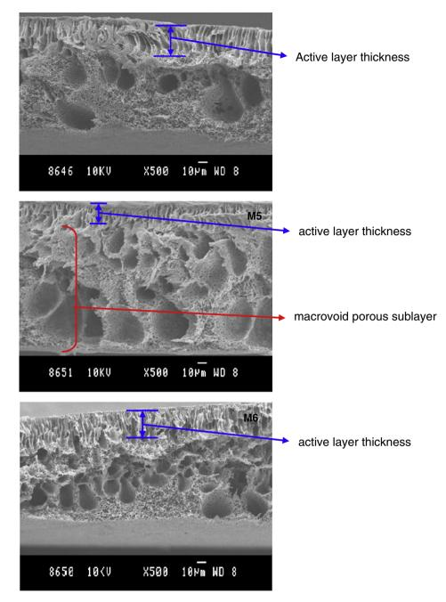
Fig. 3. SEM photographs of the cross sectional view of membranes from 85% of NMP (M4), DMSO (M5) and DMF (M6) as solvents in 15% of PES polymer, magnification 500.
