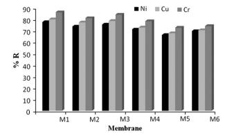
Fig. 4. Solvents effect and solvents composition in PES membranes on rejection of Cu(II), Ni(II) and Cr(III) metal ions with PVA microligand.
