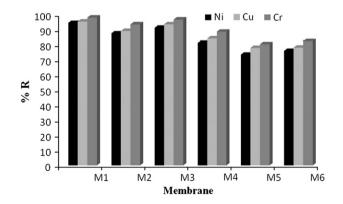
Fig. 5. Solvent effect and solvent composition in PES membranes on rejection of Cu(II), Ni(II) and Cr(III) metal ions with PDDA microligand.
