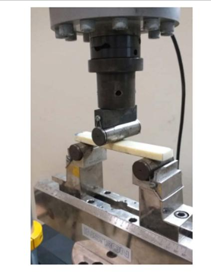
Figure 3. Bending test Instron machine.
