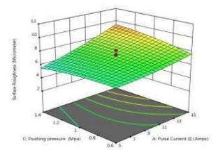
Figure 5. Effect of Roughness with Pulse Current and Pressure Flushing
