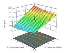
Figure. 8. MRR Vs Pulse current and pressure flushing.
