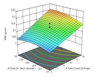
Figure .7 Effect of MRR with Pulse Direct current and Pulse time ON
