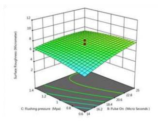
Figure 6. Effect of Roughness with Pulse time ON and Pressure Flushing
