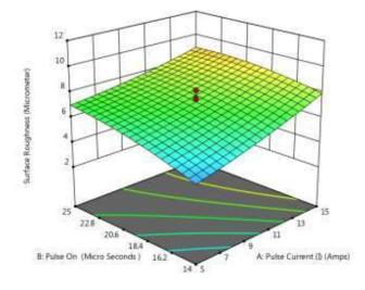
Figure 4. Effect on Roughness With Pulse Direct current and Pulse Time ON
