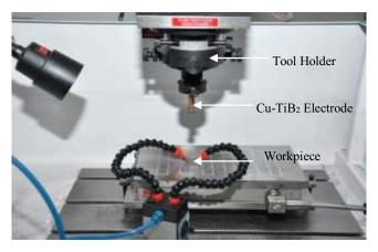
Figure 2. Set up for EDM Experiments.
