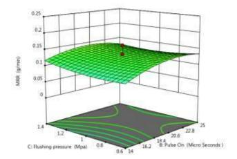
Figure. 9. MRR with Pulse time ON and pressure flushing
