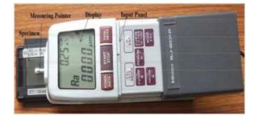
Figure 3. Surface roughness tester
