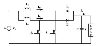
Figure 5. Interleaved boost converter (IBC) circuit diagram.
