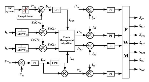
Figure 9. Control configuration of the proposed system.
