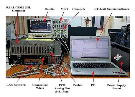
Figure 10. Real-Time (RT) results setup.
