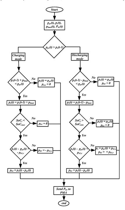
Figure 7. Power management algorithm for battery-1.
