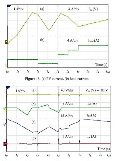
Figure 14. (a) DC link voltage, (b) battery-1 current, (c) battery-2 current, (d) super-capacitor (SC) current.
