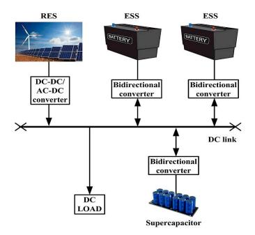
Figure 1. Typical DC microgrid (µG) system.
