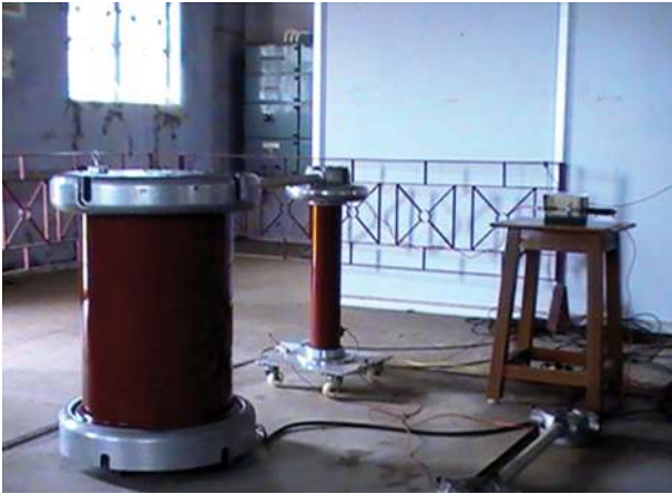
FIGURE 7: Laboratory experimental test setup indicating the direct detection PD measurement methodology.
