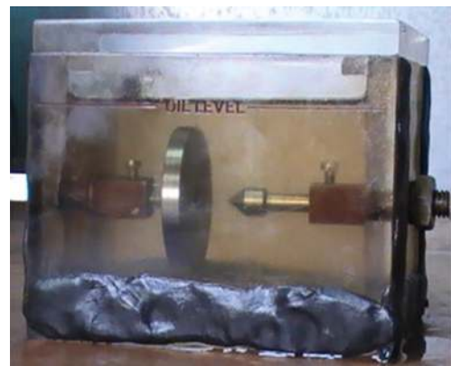
FIGURE 12: Laboratory model simulating oil corona discharge with point configuration as high voltage electrode at an 85^\circ apex angle.
