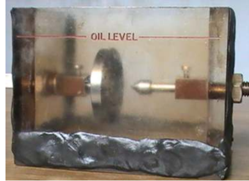
FIGURE 11: Laboratory model simulating air corona discharge with point configuration as high voltage electrode at an 85^\circ apex angle.
