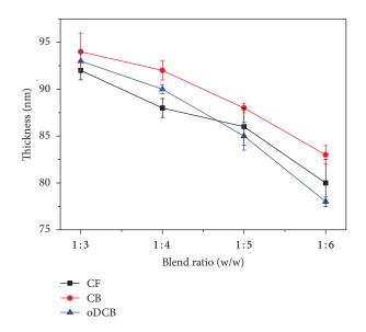
FIGURE 2: Thickness of PCDTBT:  $PC_{71}BM$  active layer films with different composition prepared in solvents of chloroform (1 wt%), chlorobenzene (2 wt%), and o-dichlorobenzene (3 wt%).
