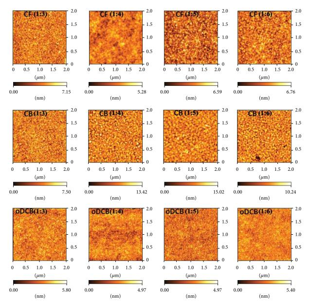
FIGURE 3: AFM images of the PCDTBT:  $PC_{71}BM$  films prepared by using organic solvents of chloroform (1 wt%), chlorobenzene (2 wt%), and o-dichlorobenzene (3 wt%): blend ratio of PCDTBT and  $PC_{71}BM$  was varied from 1:3 to 1:6.
