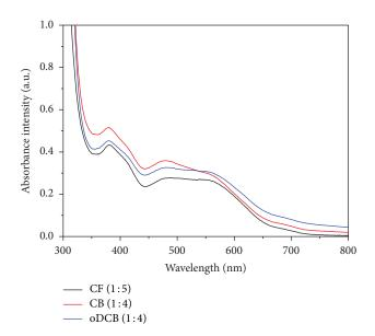
FIGURE 5: Absorption spectra of active layer of PCDTBT:  $PC_{71}BM$  prepared by using organic solvents of chloroform, chlorobenzene, and o-dichlorobenzene with PCDTBT:  $PC_{71}BM$  ratios of (1:5), (1:4), and (1:4), respectively.
