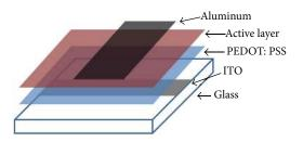
FIGURE 1: Structure of organic solar cell device with heterojunction active layer structure of PCDTBT:  $PC_{71}BM$  and buffer layer of PEDOT: PSS.
