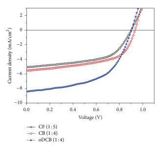
FIGURE 6: Current density (*J*)–voltage (*V*) characteristics of ITO/PEDOT :  $PSS/PCDTBT : PC_{71}BM/Al$  devices with an active layer prepared by using organic solvents of chloroform (D/A; 1: 5), chlorobenzene (D/A; 1: 4), and o-dichlorobenzene (D/A; 1: 4).
