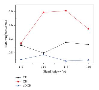
FIGURE 4: Surface roughness values obtained from the AFM images for PCDTBT:  $PC_{71}BM$  films prepared with organic solvents of chloroform (1 wt%), chlorobenzene (2 wt%), and o-dichlorobenzene (3 wt%).
