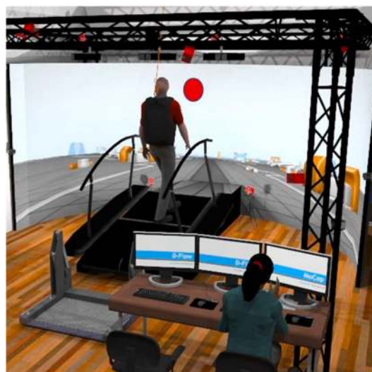
Fig. 1. Virtual Reality (VR) display with a red dot creating a forward and backward walking environment, with a treadmill belt capable of moving in two directions. (For interpretation of the references to colour in this figure legend, the reader is referred to the web version of this article.)
