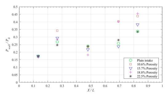
**Figure 13.** Static pressure variation along the intake-core due to wall ventilation at  $R_c = 1.19$ .
