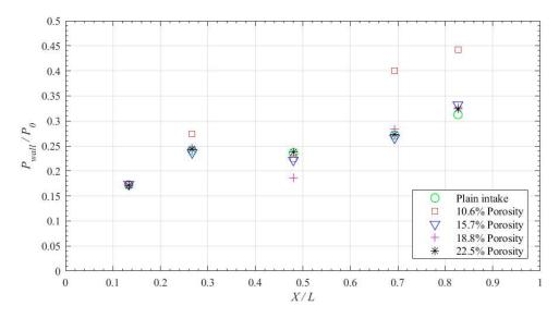
**Figure 14.** Static pressure variation along the intake-core due to wall ventilation at  $R_c = 1.22$ .
