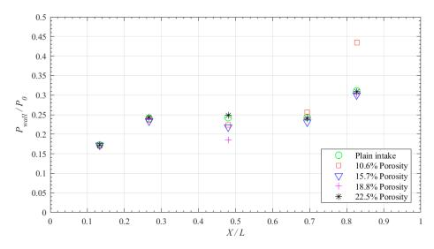
**Figure 15.** Static pressure variation along the intake-core due to wall ventilation at  $R_c = 1.25$ .
