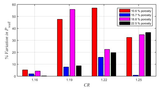
**Figure 17.** The controlled intakes with wall static pressure variations at different contraction ratios (X/L = 0.7).
