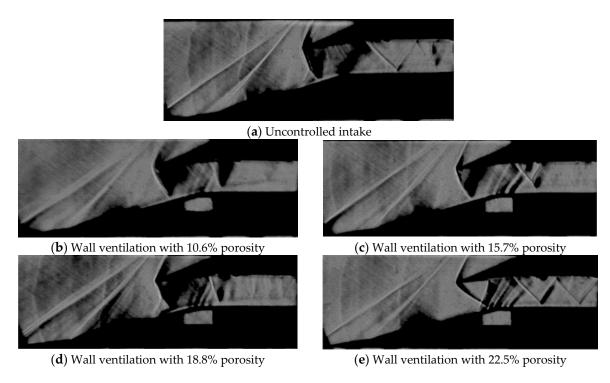
**Figure 8.** Schlieren view of uncontrolled and wall ventilated intakes at  $R_c = 1.19$ .
