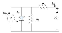
Fig.1. Schematic of One diode model.
