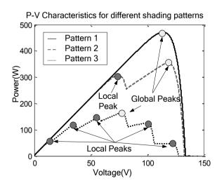
Fig.3. P-V characteristics for shade patterns
