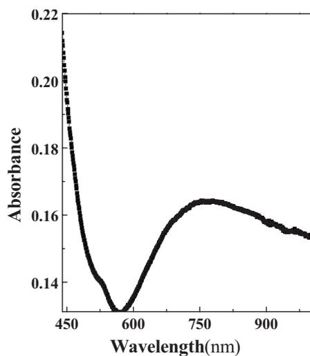
FIG. 3. UV-visible spectrum of PCz.
