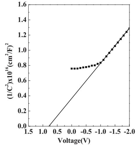
FIG. 7.  $1/C^2$  vs  $V$  characteristic of Al/PCz/ITO.
