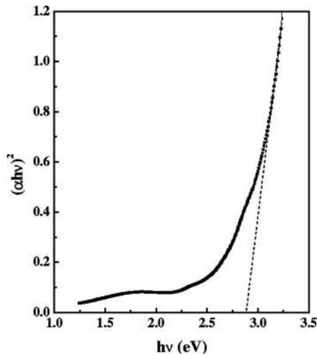
FIG. 2.  $(\alpha hv)^2$  vs  $h\nu$  plot for bandgap estimation of PCz.
