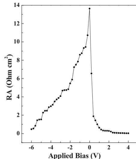
FIG. 11. Variation in  $RA$  product of the device with applied bias voltage.
