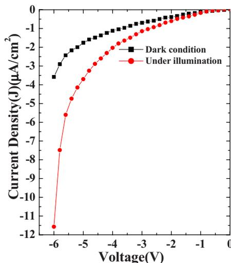
FIG. 9. (Color online) Reverse bias  $J$ - $V$  characteristics of Al/PCz/ITO under illumination of light.
