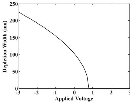
FIG. 8. Variation in depletion width ( $W_d$ ) vs applied voltage ( $v$ ).
