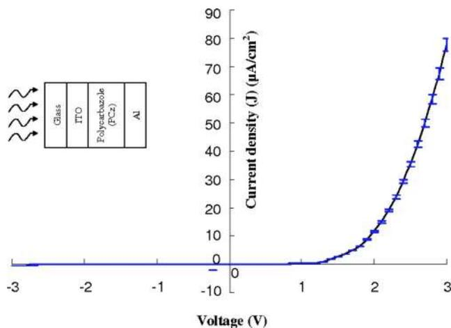
FIG. 1. (Color online)  $J$ - $V$  characteristic of Al/PCz/ITO showing standard deviation in measurements on random samples along with device configuration shown as inset.
