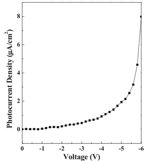
FIG. 10. Photocurrent density vs reverse bias applied voltage.
