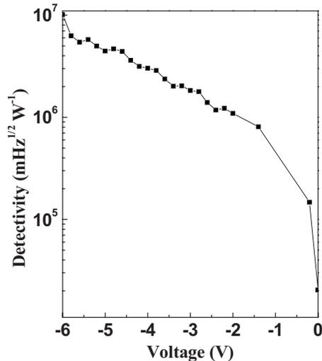
FIG. 12. Variation in detectivity of the Al/PCz/ITO with applied bias voltage.
