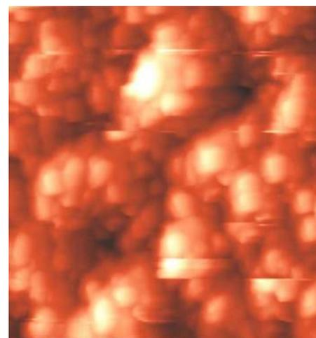
FIG. 5. (Color online) AFM image of electropolymerized PCz film on ITO coated glass substrate.
