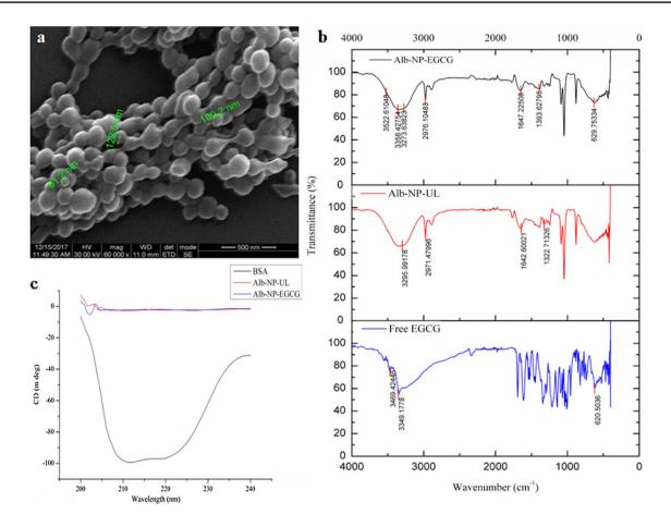
Fig. 2 Physicochemical properties of nanoparticles. a SEM image of Alb-NP-EGCG; b the FT-IR spectrum of free EGCG, Alb-NP-UL, and Alb-NP-EGCG; c circular dichroism analysis of BSA, Alb-NP-UL, and Alb-NP-EGCG
