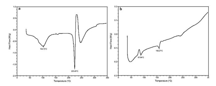
Fig. 3 Differential scanning calorimetry analysis of a free EGCG and b Alb-NP-EGCG
