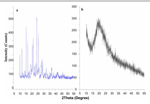
Fig. 4 X-ray diffraction (X-RD) analysis of a free EGCG and b Alb-NP-EGCG
