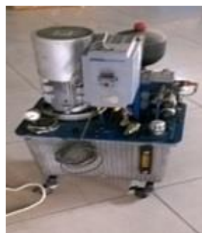
Figure 2: Hydraulic power pack
