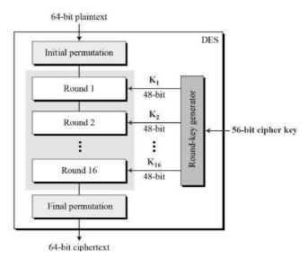
Fig. 7. Data Encryption Standard Architecture
