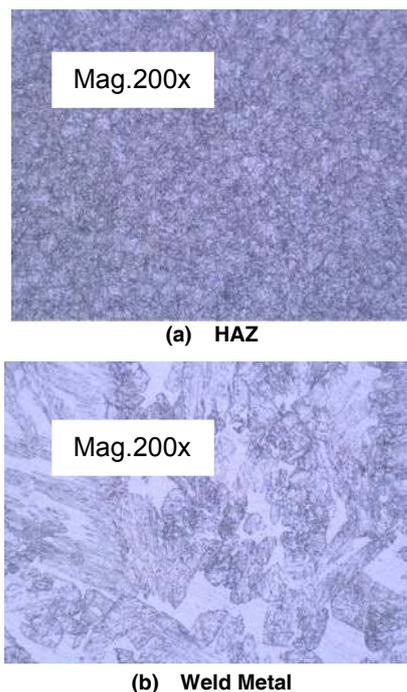
Figure 4: Microstructure of Argon gas specimen HAZ & WM
