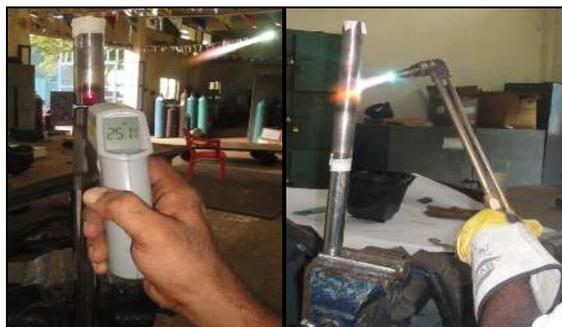
**Figure 1: Pre heating the test specimen**
