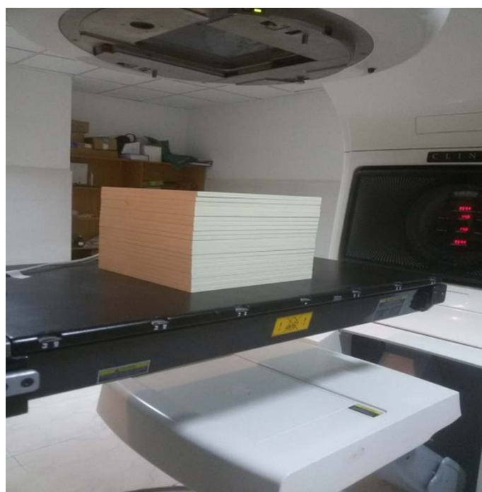
Figure 1. Experimental setup for Gy/CU table generation
