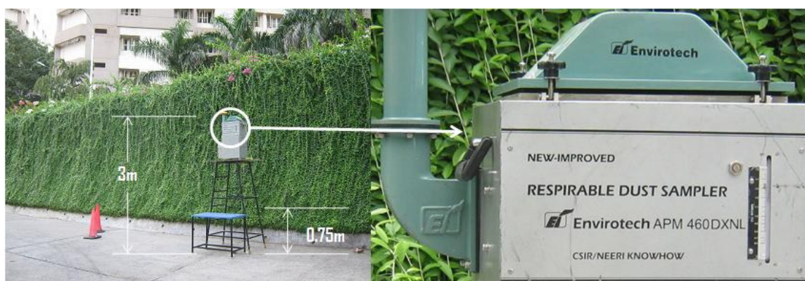
Figure 13: Particulate matter and gaseous sampling in the subway on 29th July 2013, using Envirotech APM4 60DXNL with APM411.
