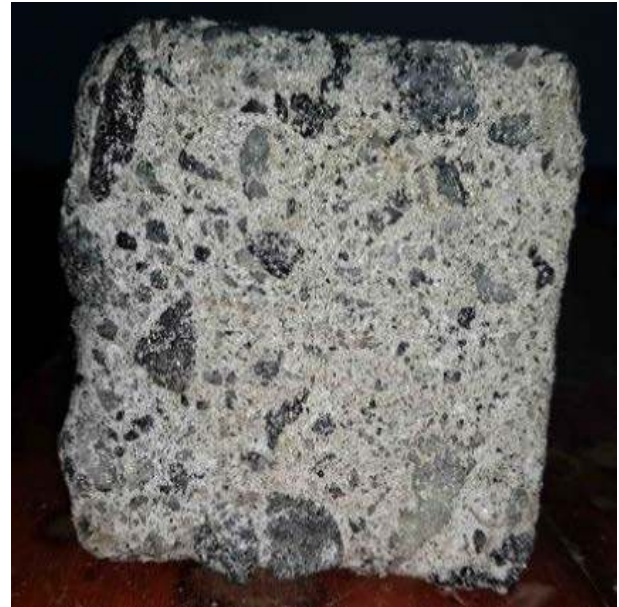
Figure 8(c). The Acid Attacked Specimens at 28 days with 20% CPA
