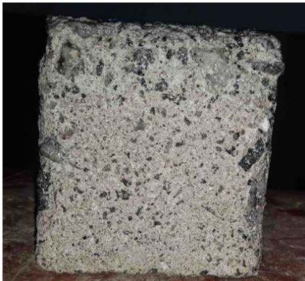
Figure 8 (b). The Acid Attacked Specimens at 28 days with 10% CPA
