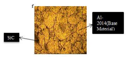
Fig. 8 Surface Morphology for Sample 2
