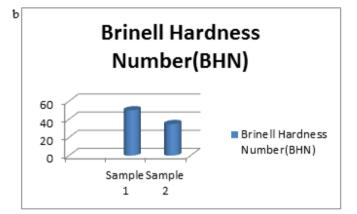
Figure 3 shows the Brinell hardness values for two different reinforced brake pad materials
