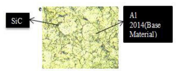
Fig. 7 Surface Morphology for Sample 1
