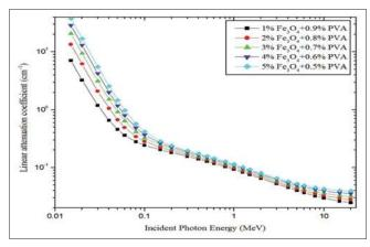
Figure 2: Linear attenuation coefficient for different polymer composite materials plotted against incident photon energy
