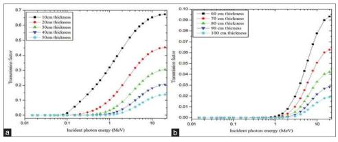
Figure 6: (a and b) Transmission factors for different thicknesses of polymer composite with 0.5% of magnetite plotted against incident photon energy
