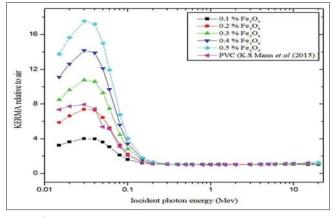
Figure 8: kinetic energy released per unit mass relative to air plotted against incident photon energy
