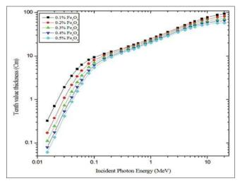
Figure 5: Tenth-value layer for different polymer composite materials plotted against incident photon energy
