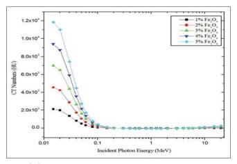
Figure 3: Computer tomography number for different polymer composite materials plotted against incident photon energy
