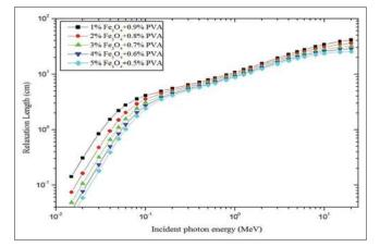
Figure 7: Relaxation length for concentrations of magnetite plotted against incident photon energy
