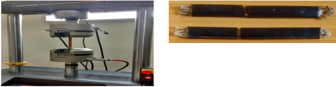
Figure 3. Tensile Testing and fractured specimens.
