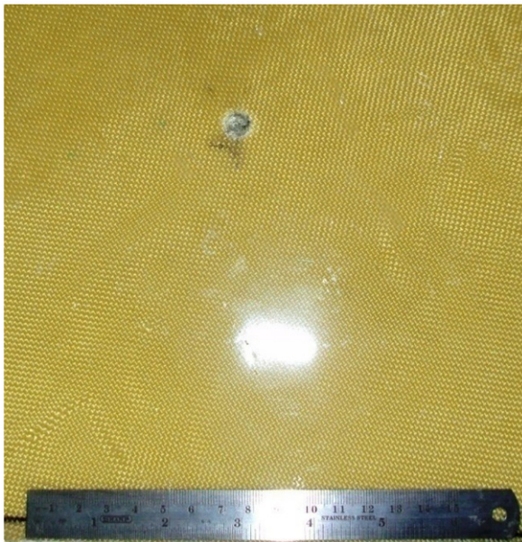
Figure 3. Damage area at front face of 0/90.
