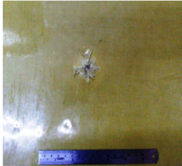
Figure 9. Damage on rear side of 19 layers 0/90 plate.
