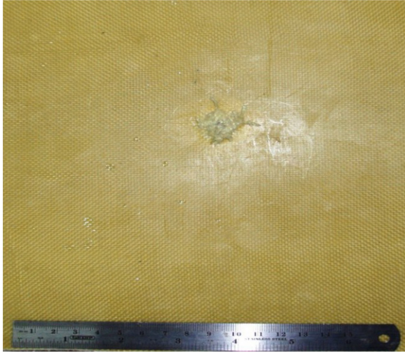
Figure 11. Damage on rear side of 12 layers 0/90 plate.
