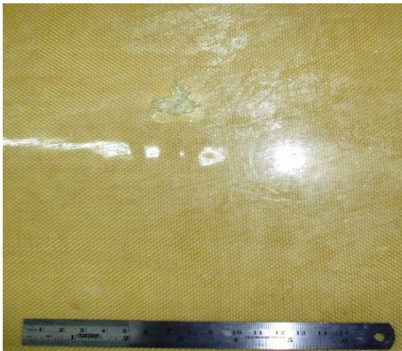
Figure 12. Damage on rear side of 8 layers 0/90 plate.
