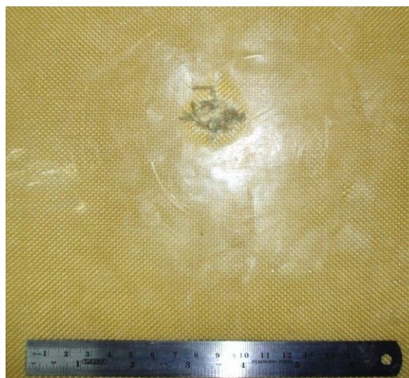
Figure 10. Damage on rear side of 15 layers 0/90 plate.
