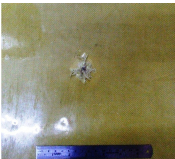
Figure 5. Damage at rear face of 0/90, 19 layer laminate.
