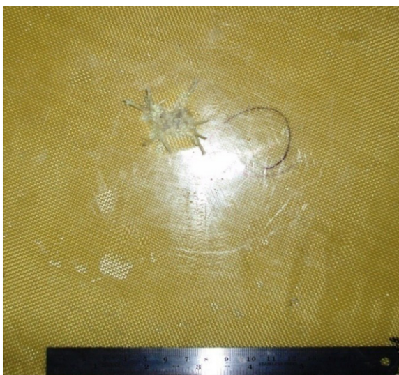
Figure 8. Damage on rear face of 30/60/30/60 19 layer laminate.
