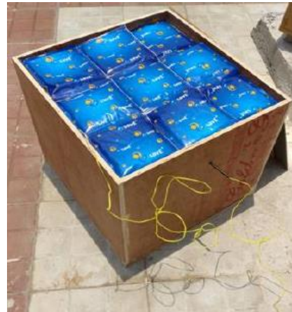
Figure 2. Storage box with PCM.
